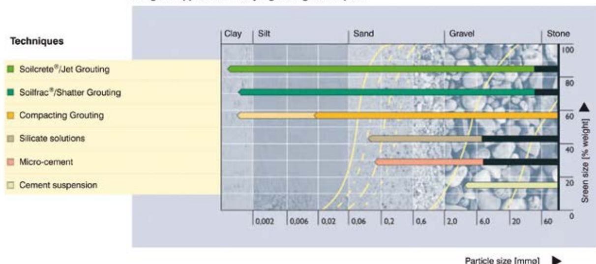
Range of applications for jet-grouting techniques
